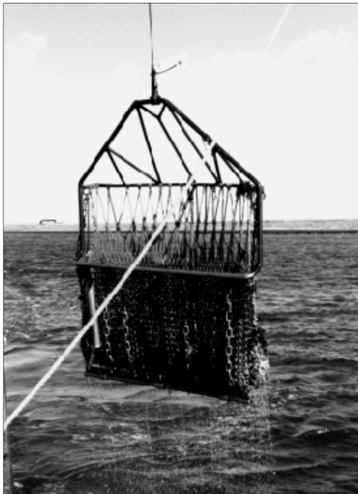
Figure 1 The dredge-net used for the collecting of fossils; the attached metal pipe is clearly visible. (photo: J.W.F. Reumer)
